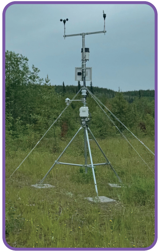
Figure 2. The established climate monitoring station installed as part of the project tracks rainfall, temperature, and wind patterns affecting forest service roads.
